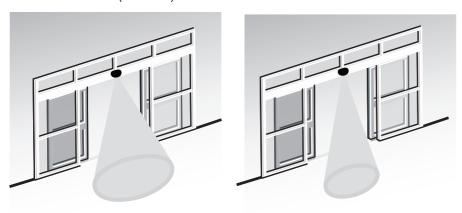
The size of the detection area can be changed using the potentiometer.
